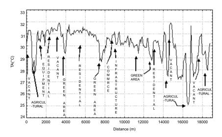
Fig. 9. Thermal profile (transect 2, NE-SW) extracted from Figure 8.
