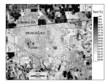
Fig. 7. Spatial distribution of Estimated air temperature (°C) from Landsat thermal image (May/12/2003-10:00 a.m. local time). Brighter tones represent higher temperatures.
