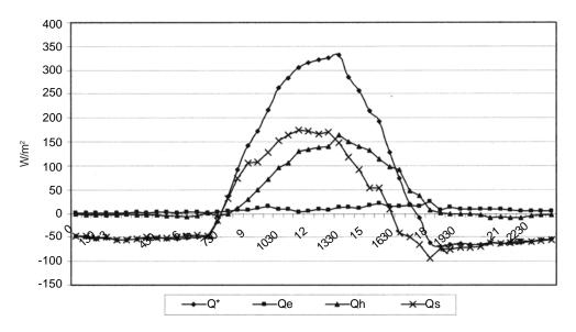
Fig. 4. Behavior of the atmospheric energy balance in the surface layer from 18-22 February, 2001. Q\* (net radiation), Q<sub>e</sub> (latent heat), Q<sub>h</sub> (sensible heat), Q<sub>s</sub> (heat stored in the near layer).
